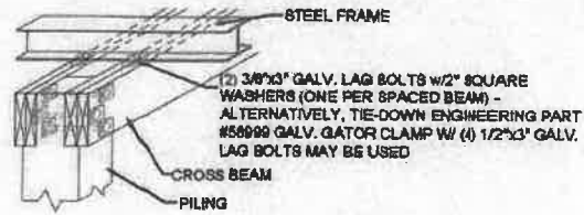
FRAME CONNECTION DETAIL
